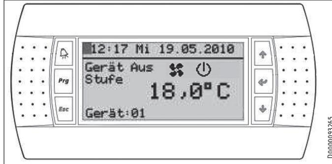
The unit's programming unit comprises a display and 6 buttons. The "Alarm" button reports accumulated fault and maintenance messages by permanently illuminating or flashing red. The "Prg" button illuminates orange when performing entries on the programming unit; the other buttons illuminate green.
